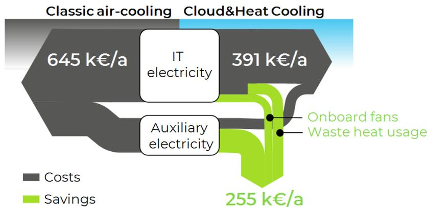
Illustration 5: Cost flow diagram - standard air-cooling vs. Cloud & Heat Cooling
