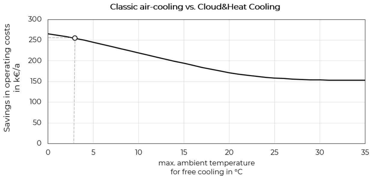
*Illustration 6: Potential savings in operating costs, in relation to the maximum ambient temperature<sup>16</sup> at which free cooling is possible - classic air cooling vs. Cloud&Heat Cooling*
